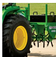
Core Aerator Keep grass roots healthy. Allows oxygen in the ground and opens the soil to accept fertilizer.
